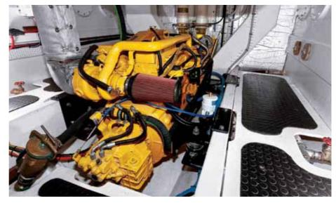
In fact, he designed the engine room to fit the PowerTech 6068TFM engine. "The engine room on *Stormboy* is large by pleasure boat standards, and the engine fit in easily, low in the keel, with an almost straight shaft angle. All of the important bits on the engine are easily accessible," comments Jim.
